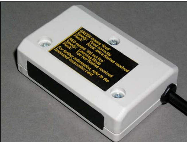
Bottom view of the completed unit. The infrared window is to the left
