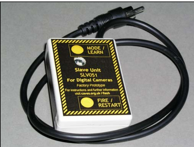
A view of the completed unit. The infrared window is to the left
